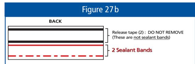
\*Manufactured in the West. Sealant Bands are located on the Top / Front of each Shingle (also see Figure 27a).
