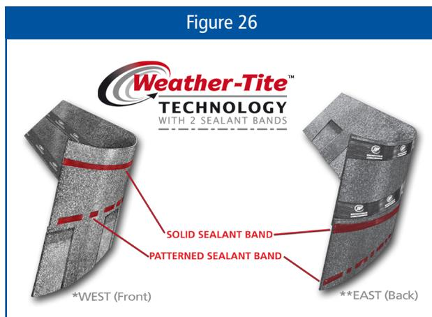
Mystique 42, Vanguard 42 IR and Manoir laminate shingles have 2 sealant bands located on the front of the shingle as well as 2 release tapes (to prevent sticking during stacking) on the back which should not be removed (see Figure 27a).
