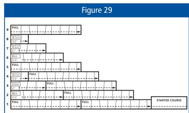
53.3 cm (21") from the left end of the shingle and apply the long section over the headlap of the second course. Begin the fourth course with a partial shingle measuring 26.7 cm (10.5") establishing the overall diagonal method. Start the fifth course with a full shingle, repeating the process beginning with a full shingle and starting each succeeding course as described above. Continue to make your way across the roof, ensuring a 15.2 cm (6") exposure throughout the roof (see [Figure 29](#)).
