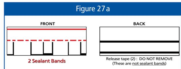
Mystique 42 and Everest 42 laminate shingles have 2 sealant bands as well as 2 release tapes (to prevent sticking during stacking) on the back which SHOULD NOT BE REMOVED (see Figure 27b).
