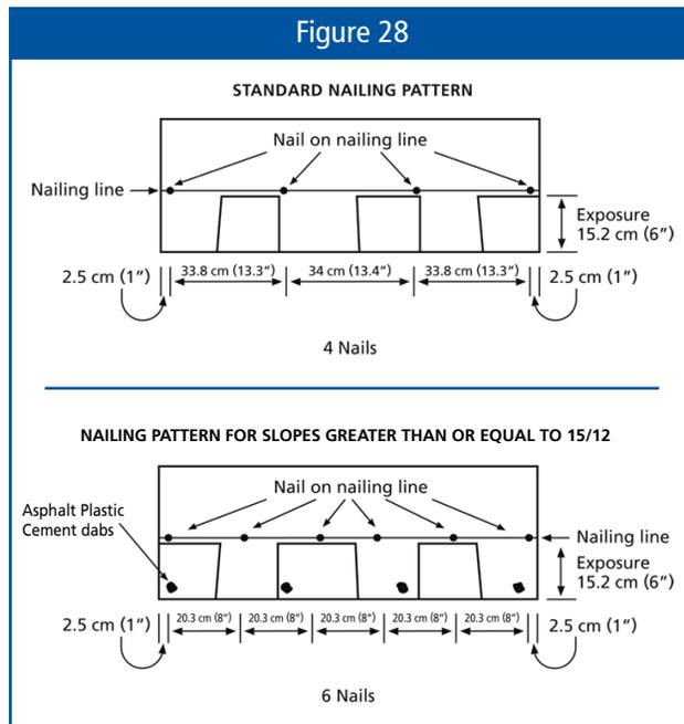
Everest 42 and Mystique 42 shingles must be nailed on the nailing line to allow penetration through the double-ply area just above the tops of the laminated tabs. Nails must be long enough to penetrate a minimum of 19 mm ( $\frac{3}{4}$ " ) into solid wood deck or just through the plywood deck.
