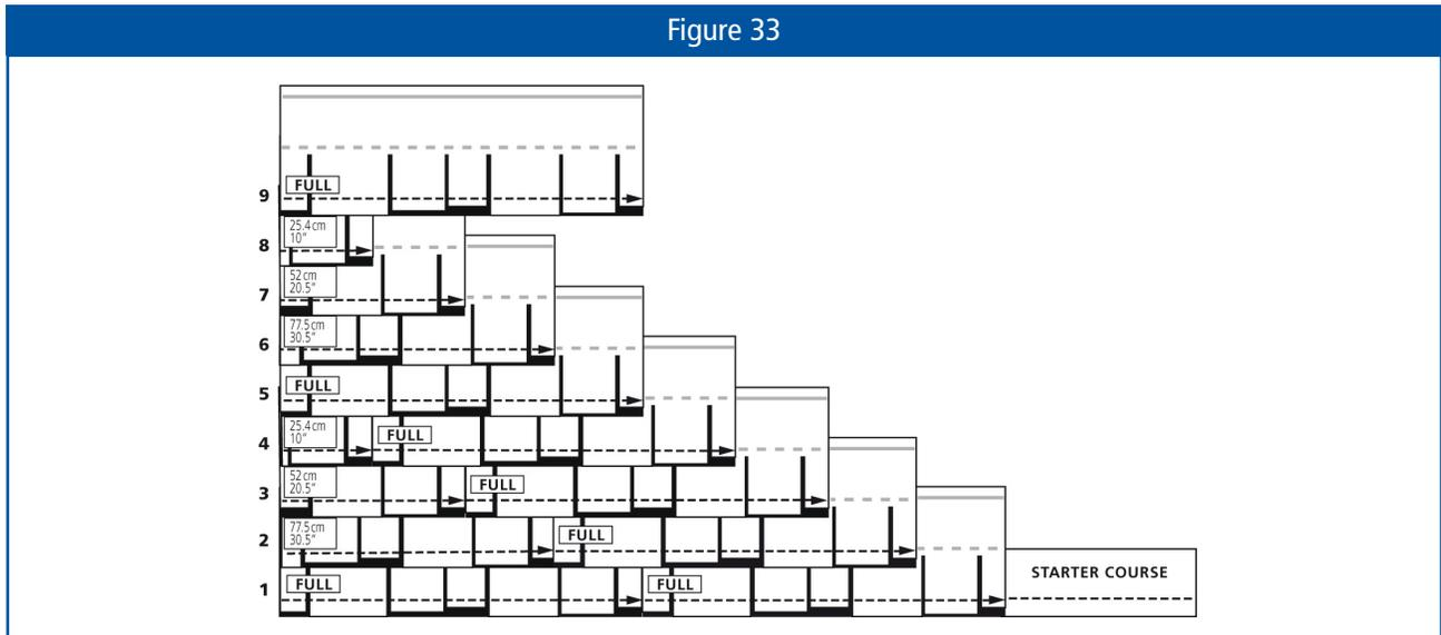
**NOTE :** When working with cut piece, ensure that there is a minimum of 15.2 cm (6") offset between the ends of pieces from row to row. Always leave a space of 1" minimum between the nail heads and the shingle edges.
